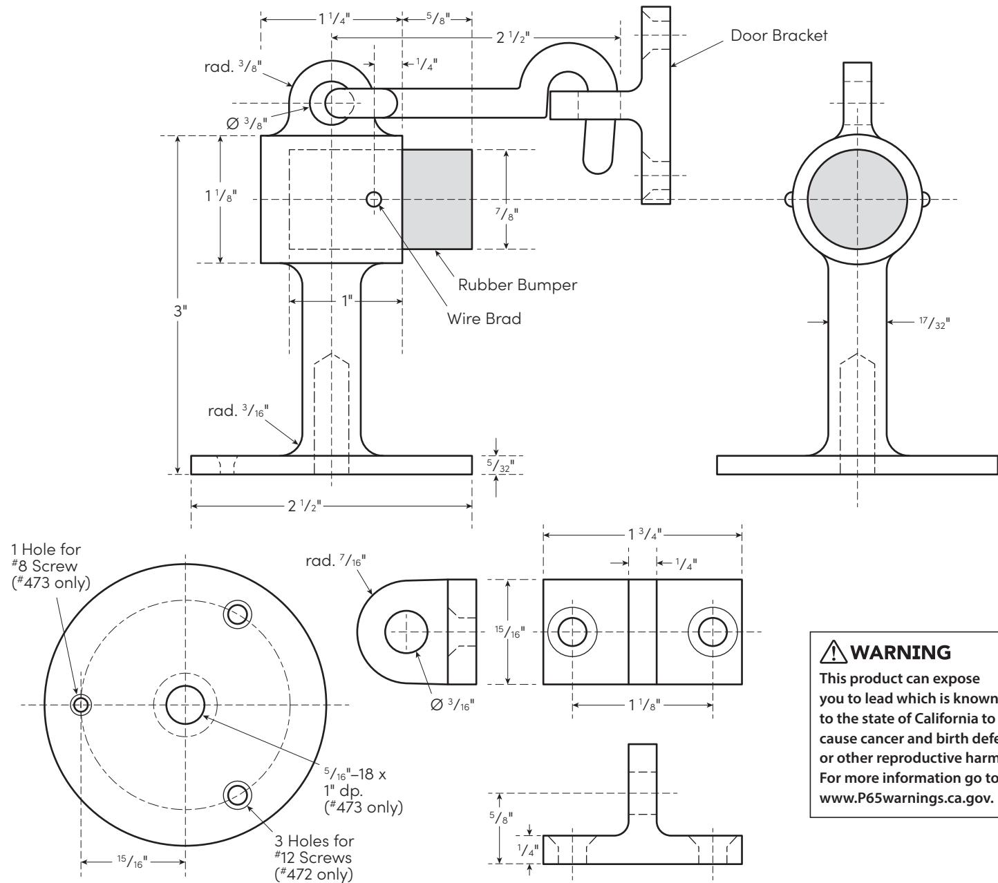
**MATERIAL:** Cast Brass with Rubber Bumper**FASTENERS NOTE:** Stop:  $5/16\text{"-}18 \times 1\frac{3}{4}\text{"}$  Stud, Anchor (Prep for Anchor -  $5/8\text{"}$  drill bit);
