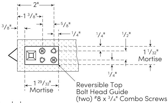
Reversible Top Bolt Head Guide (two) #8 x 3/4" Combo Screws
